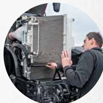
Fast and simple cleaning of the radiator and air-conditioning system.
