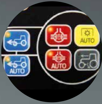
Automatic all-wheel drive and differential lock management
