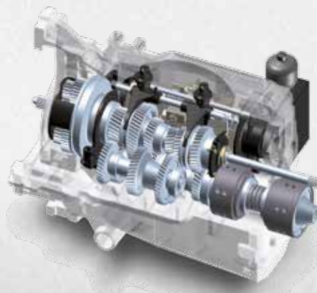
Continuously variable transmission from 0 to 50 km/h.
